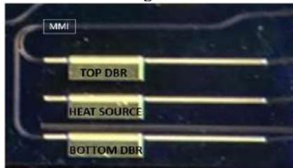
Figure 1: Picture of the Photonic Integrated Circuit.
